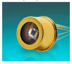
Real-time measurements are easily supported with BXT2S-28T's fast response time. The cooled unit delivers additional sensitivity for very low-level signal detection and enhanced stability for harsh environments where temperatures are in constant flux. It offers consistently high performance in gas analysis and monitoring tasks, which are key to vital medical, defense, and industrial applications.
