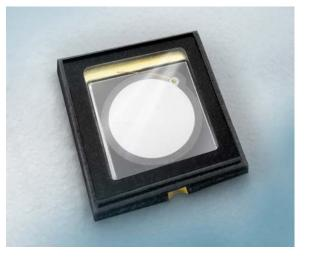
The NIR-enhanced detector is specially designed for laser monitoring, medical diagnostic equipment, industrial automation, scientific measurement, and military applications which require a wide operating temperature range from -40 degrees C to +125 degrees C. The robust package features an AR-coated window that provides greater than 98% transmission. The SMD is compliant with RoHS and REACH standards and is available on tape and reel.
