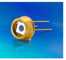
Electro-optical characteristics include responsivity at 0.09 A/W (minimum) to 0.115 A/W (typical) and dark current of 1nA. The reverse breakdown voltage ranges from 25 V (minimum) to 50 V (typical), and capacitance is 500 pF (minimum) to 1500 pF (maximum). Response time is 1  $\mu$ s (minimum) to 2  $\mu$ s (maximum).
