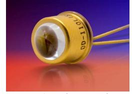
(typical), and features a storage and operating temperature of -65 °C to +150 °C. Peak emission wavelength is 880 nm with a spectral bandwidth of 55 nm (typical). The half intensity beam angle is 7 degrees (typical). The forward voltage is from 1.75 volts (typical) to 2 volts (maximum) with reverse breakdown voltage ranging from 5 volts (minimum) to 30 volts (typical). Other features include rise and fall times of 20 nanoseconds, respectively.
