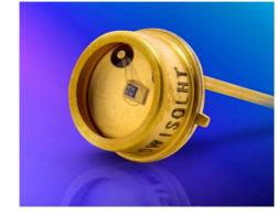
half intensity beam angle of 110 degrees and is conveniently packaged in a 2-lead TO-39 can with an isolated case. Forward voltage is 1.75 volts (typical) to 2 volts (maximum); reverse breakdown voltage ranges from a minimum of 5 volts to 30 volts (typical). The rise and fall times for the high-temperature wide angle IRLED is 20 nanoseconds, respectively.
