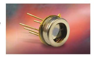
The new photodiode features excellent responsivity providing 0.125 to 0.02 A/W over a 10 to 200 nm wavelength range. The large circular detection surface is optimized for precise alignment of lasers with 4 elements, each offering 1.25 mm<sup>2</sup> active area. The compact TO-5 package allows for easy integration into new or existing systems.
